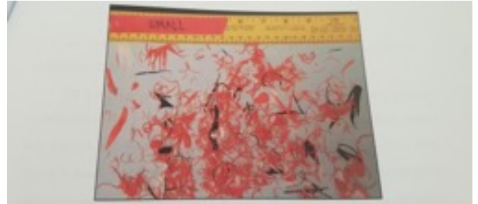
Fig. 5. Small balloon fragments (9.1% total weight released) recovered after rupture in upper atmosphere
