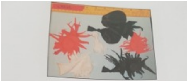
Fig. 3. Large balloon fragments (81.85% total weight released) recovered after rupture in upper atmosphere
